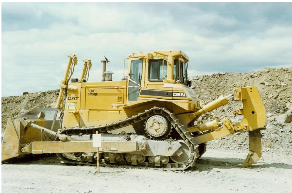
Figure 4-1 Illustration of equipment for ripping technique [RD27]
